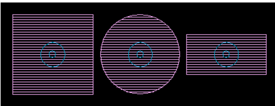
User defined Via and Route keepouts added to pins or holes
