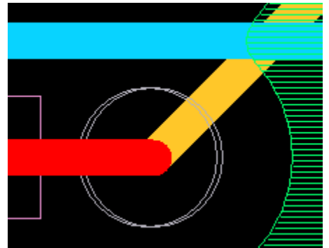
Duplicate via with less than 1 thou offset
