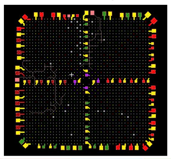
58 DISCRETES connected under the BGA sharing 116 VIAS.
