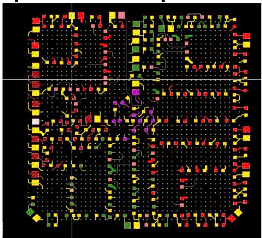
183 DISCRETES connected under the BGA sharing 366 VIAS compared to 116.
