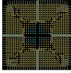
Notice the 45 degree routing required to utilize the corners. Also 5 between in "plus sign/cross".
