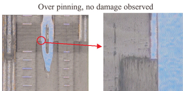
No evidence of delamination at the interface of plate hole and back drilled hole
